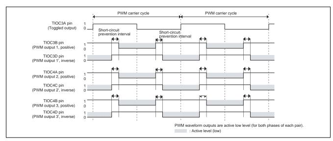
Figure 4 Output Waveforms in Complementary PWM Mode Operation
