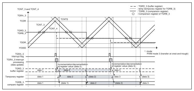
Figure 7 Timing of Updating the PWM Duty Cycle
