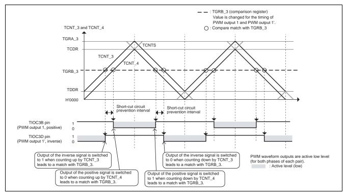
Figure 6 Output of PWM Waveforms in Complementary PWM Mode
