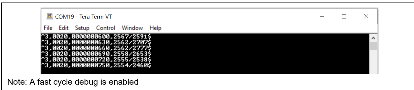
Figure 45. Example of Data Output Triggered by Analog Level Judgment Result
