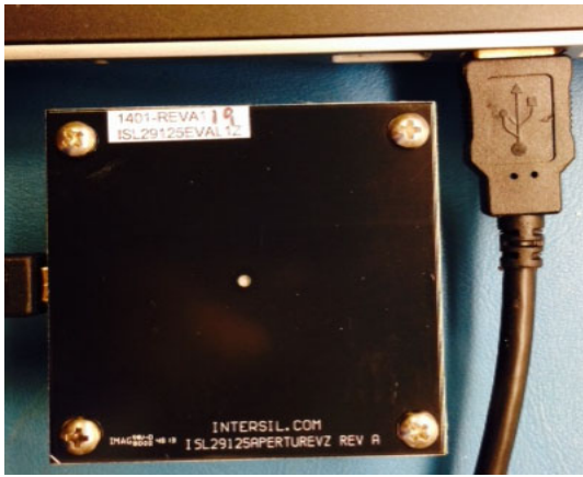
FIGURE 7. ISL29125 EVALUATION BOARD CONNECTED TO PC BY MINI USB
