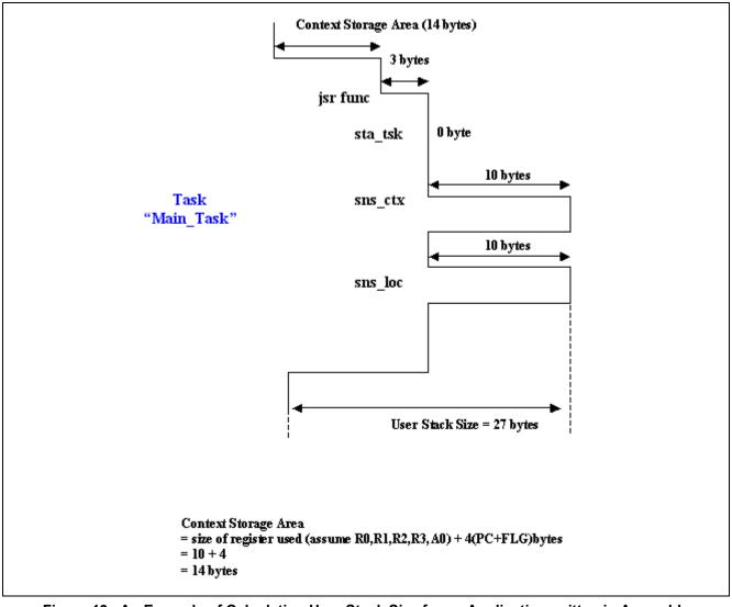
Figure 13 An Example of Calculating User Stack Size for an Application written in Assembly Language
