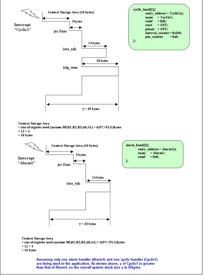
Figure 23 An Example of Computing  $\gamma$  for Application Written in Assembly Language
