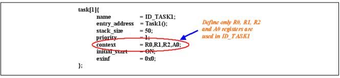
Figure 12 Task Definition in Configurator File
