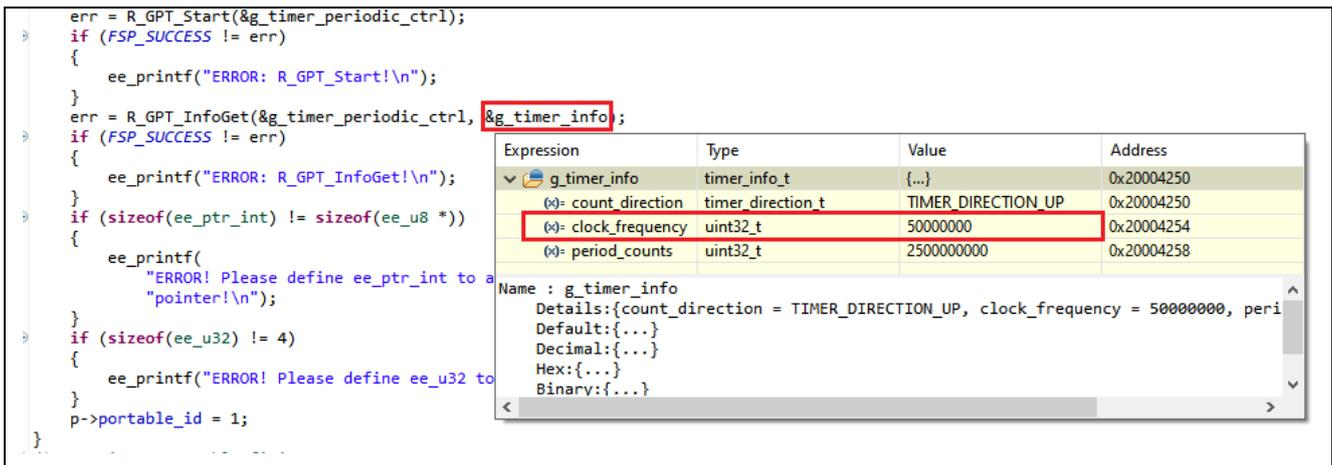
Figure 25. Check CLOCK\_PER\_SEC Setting
