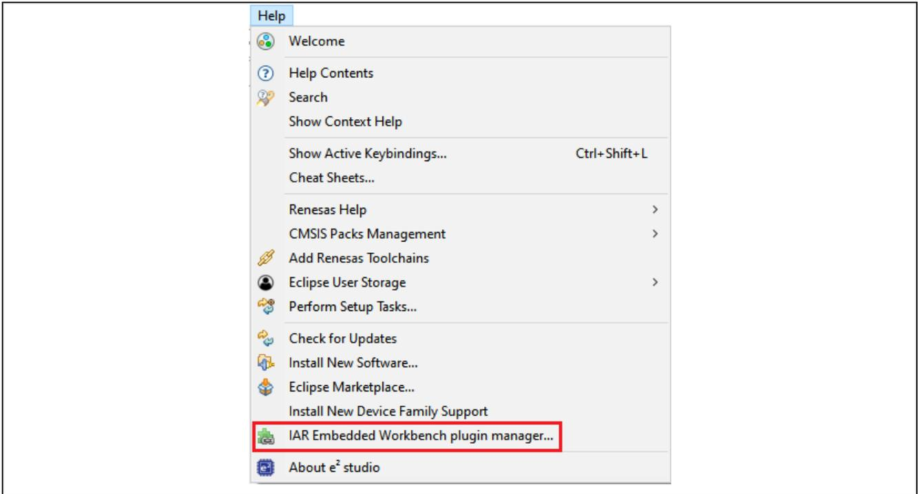
Figure 1. Select IAR Embedded Workbench Plugin Manager
