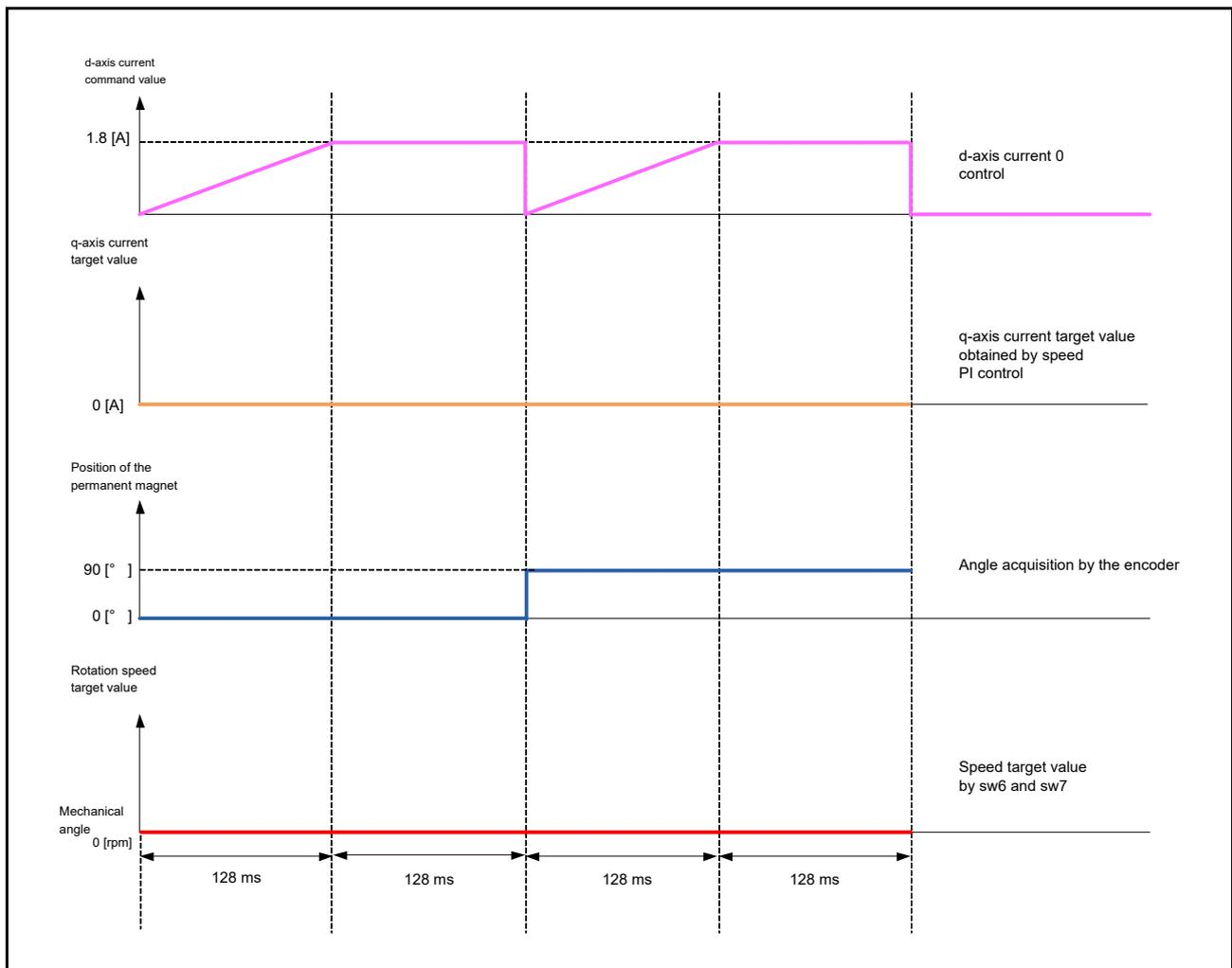
Figure 3.5 Motor Start Control
