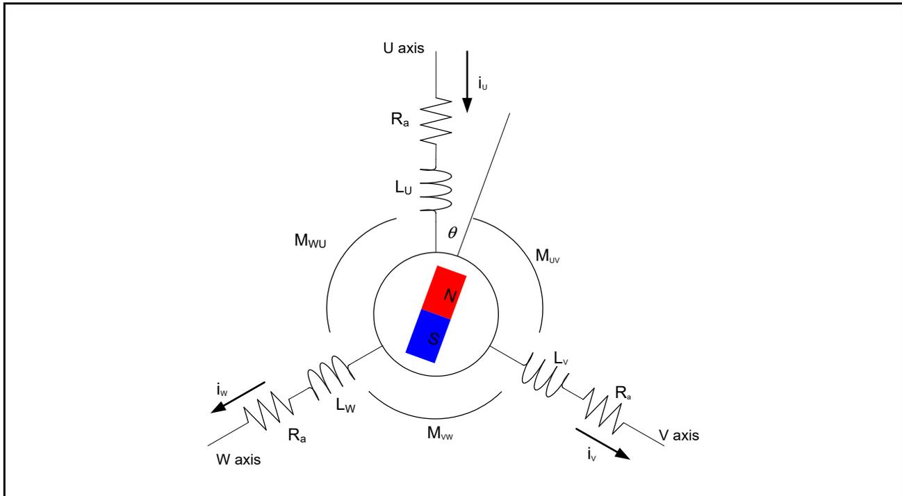
Figure 3.1 Conceptual Diagram of the 3-Phase Permanent Magnet Synchronous Motor
