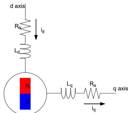
Figure 3.2 Conceptual Diagram of the 2-Phase DC Motor
