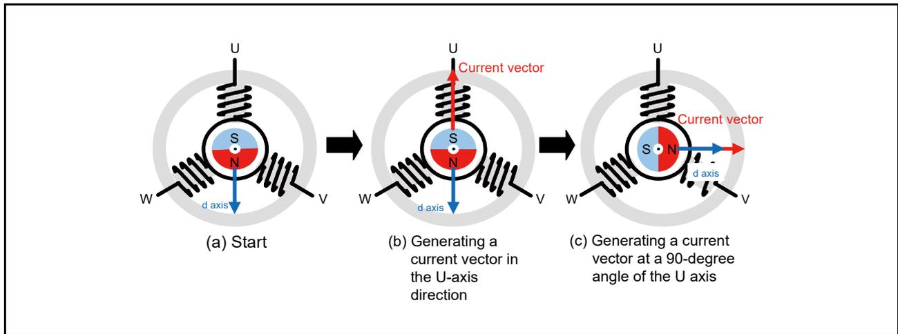
Figure 3.4 Determining the Position of the Permanent Magnet
