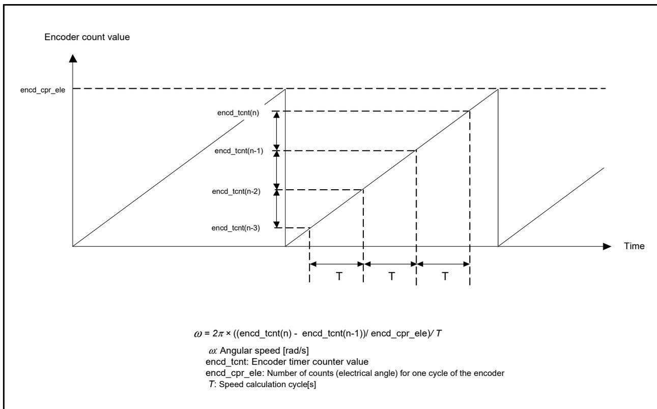
Figure 3.6 Calculating the Speed by Using the Encoder
