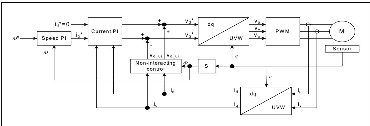
Figure 3.3 Control Flow of Vector Control
