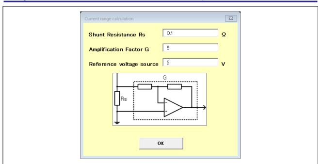
Figure 2-10 "Current range calculation" window
