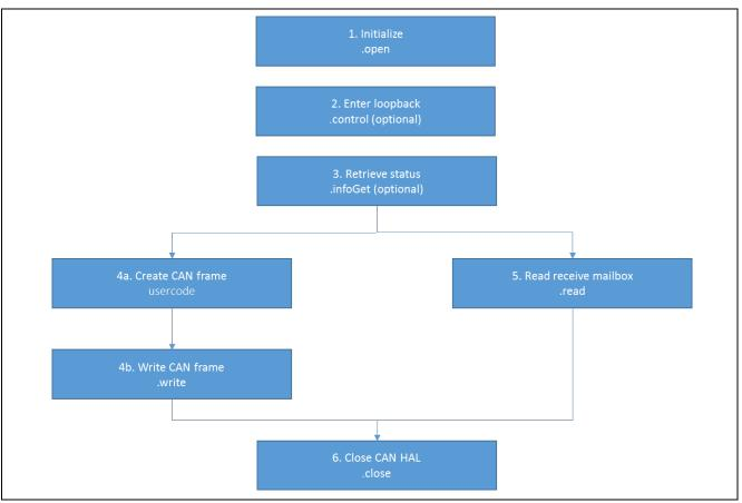
Figure 3 Flow Diagram of a Typical CAN HAL Module Application
