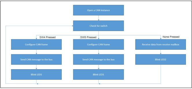
Figure 4 CAN HAL Module Application Project Flow Diagram
