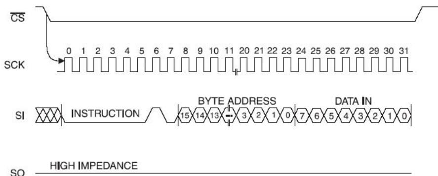
**Figure 2-6. PROGRAM command Timing (AT25Fxxxx).**
