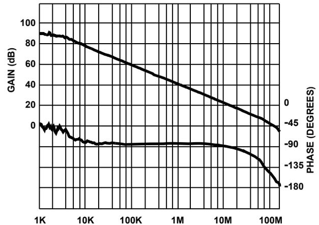
FIGURE 18. OPEN LOOP FREQUENCY RESPONSE OF THE HA2842C
