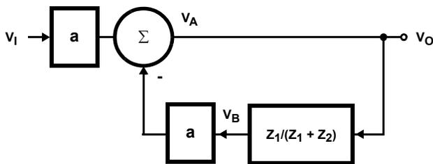
FIGURE 4A. BLOCK DIAGRAM AS WRITTEN FROM EQUATION 12
