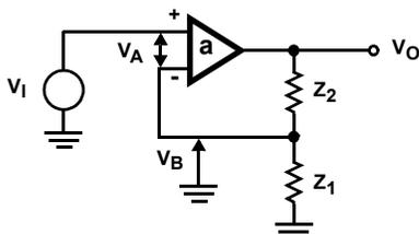
FIGURE 3. NON-INVERTING CIRCUIT
