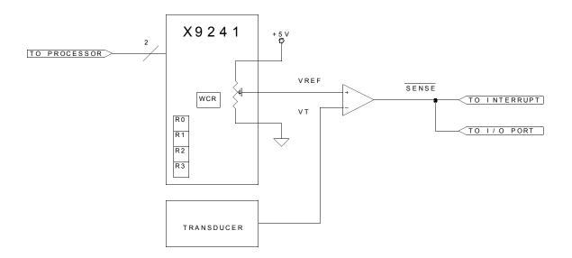
FIGURE 2. SMART MONITOR USING X9241 QUAD XDCP
