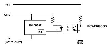
FIGURE 6. NEGATIVE VOLTAGE APPLICATION DIAGRAM
