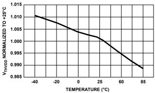
FIGURE 2. NORMALIZED OVER-TEMPERATURE V<sub>THVDD</sub>
