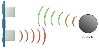
Figure 4. Operation of the ultrasonic sensor
