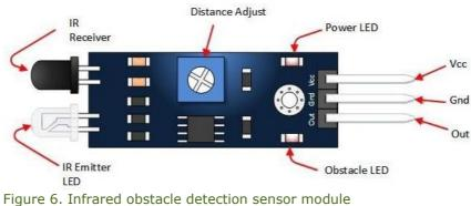
Figure 6. Infrared obstacle detection sense
