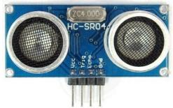
Figure 3. The HC-SR04 ultrasonic sensor
