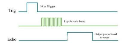
Figure 5. Trigger and Echo signals
