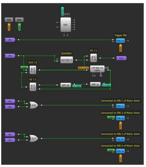
Figure 10. GPAK configuration (Matrix 1) of obstacle avoidance robot
