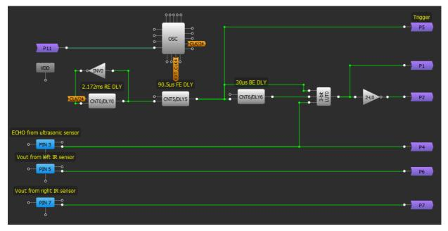
Figure 9. GPAK configuration (Matrix 0) of obstacle avoidance robot
