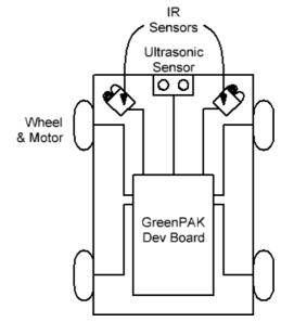
Figure 1. Autonomous Vehicle Design
