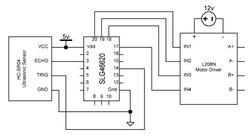
Figure 8. Block diagram showing the connections
