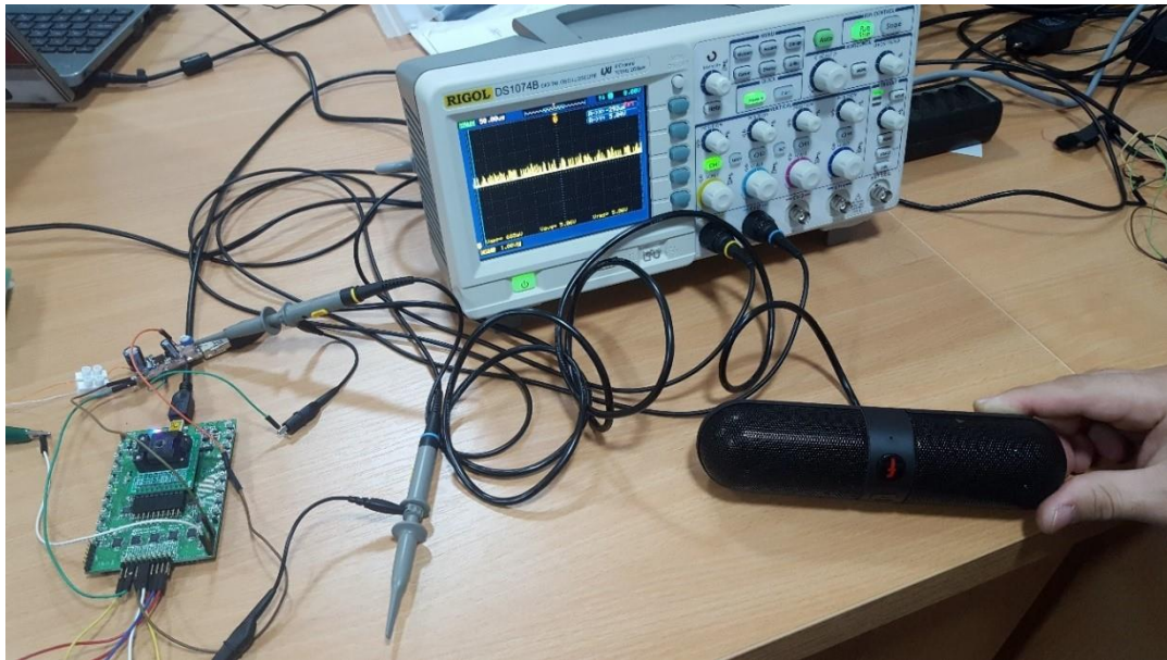
Figure 26. Boost implementation test charging Bluetooth speaker
