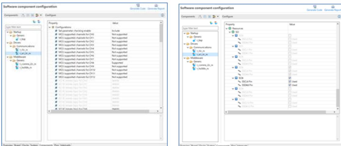
Open the "Pins" tabbed page and check that functions are assigned to the SCI8 pins in the "Pin function" panel.
