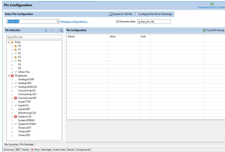
If the desired board is not displayed in the drop-down list for "Select Pin Configuration", click on [Manage Configuration] to open the "Manage Pin Configuration" window and select the desired board in the window.
