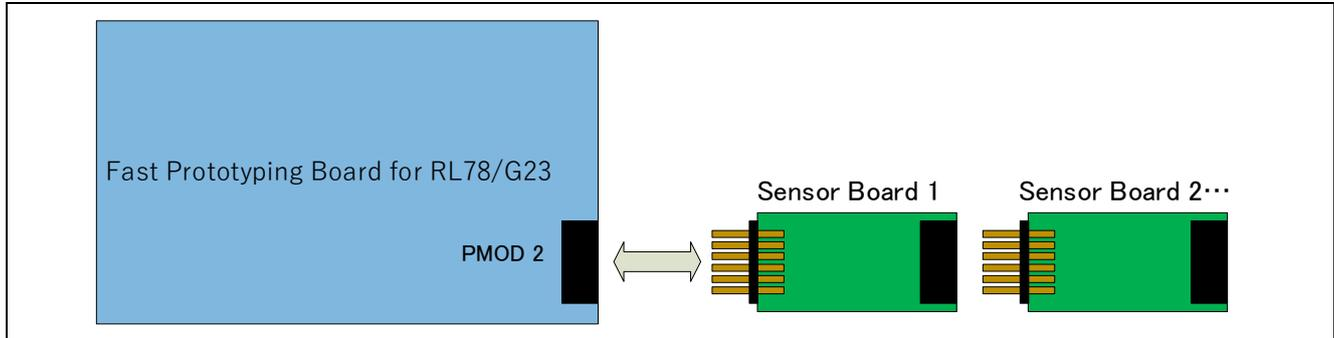
Figure 2-4 Hardware Connections for the RL78/G23 Group
