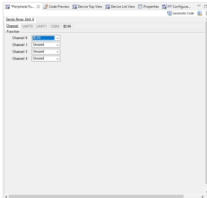
In the tabbed page for IICxx enabled in the serial array unit, set "Transfer rate" to 400000 or 100000, set "Transfer end interrupt priority" to a desired value, and enable all functions under "Callback function setting".
