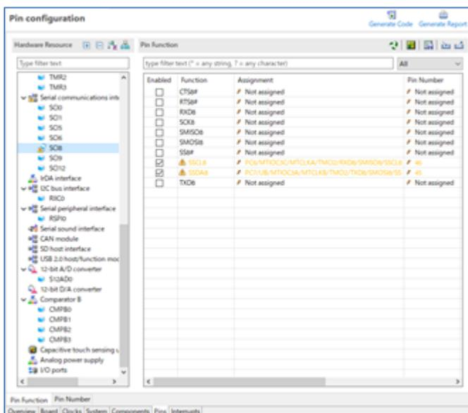
As the use of PMOD Type 2A (extended SPI) is specified in the RSK RX231 board information, a warning message will appear when I2C is used, but this does not produce any problems.
