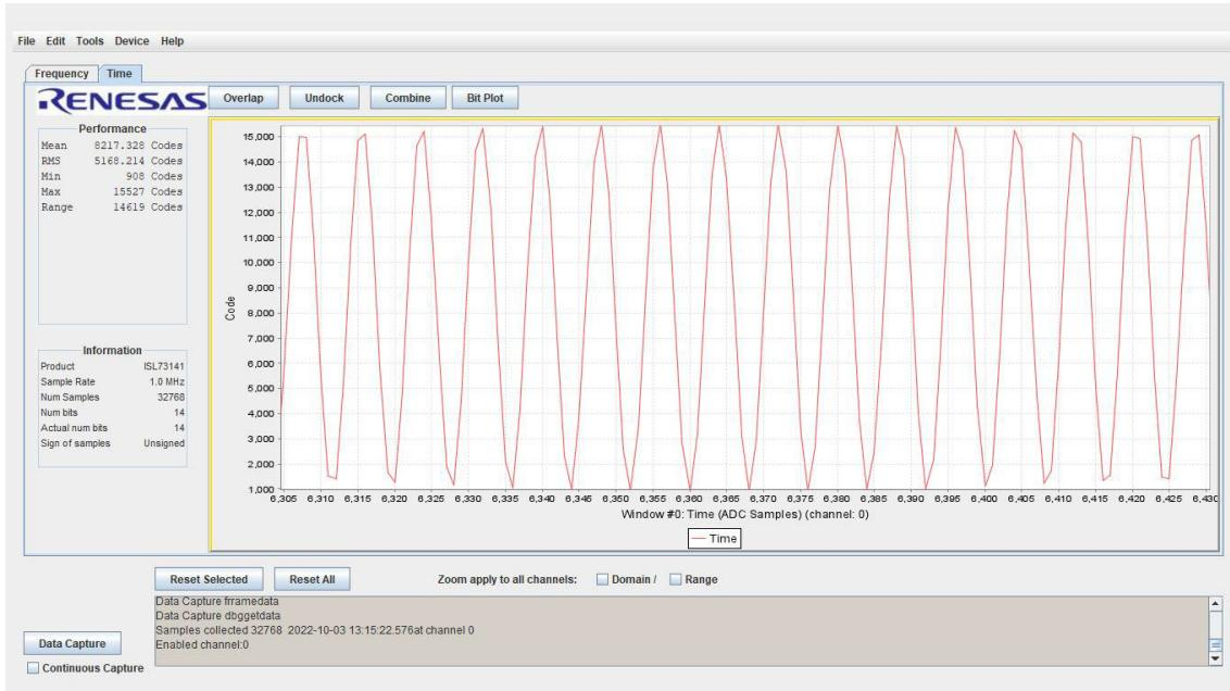
**Figure 8. iRADAnalyzer Time Domain Plot (New Image)**
