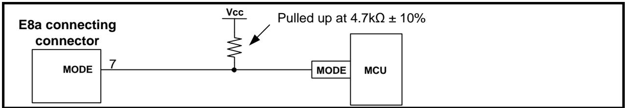
Figure 4.2 E8a Emulator and MODE Pin Connection
