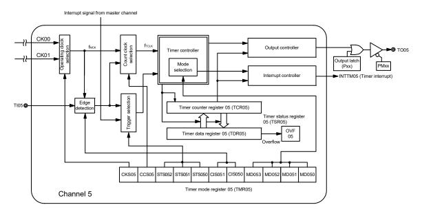
Figure 6 - 6 Internal Block Diagram of Channel 5 of Timer Array Unit
