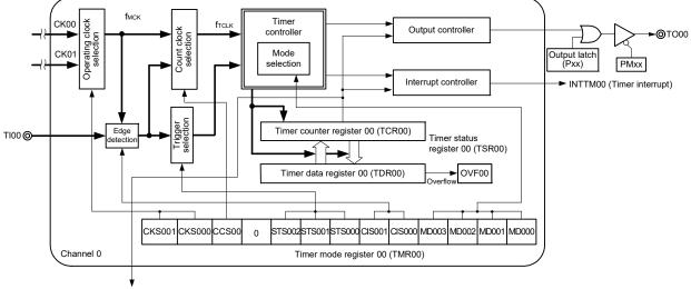
Figure 6 - 2 Internal Block Diagram of Channel 0 of Timer Array Unit
