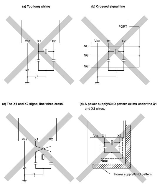
NoteDo not place a power supply/GND pattern under the wiring section (section indicated by a broken line in the figure) of the<br/>X1 and X2 pins and the resonators in a multi-layer board or double-sided board.<br/>Do not configure a layout that will cause capacitance elements and affect the oscillation characteristics.
