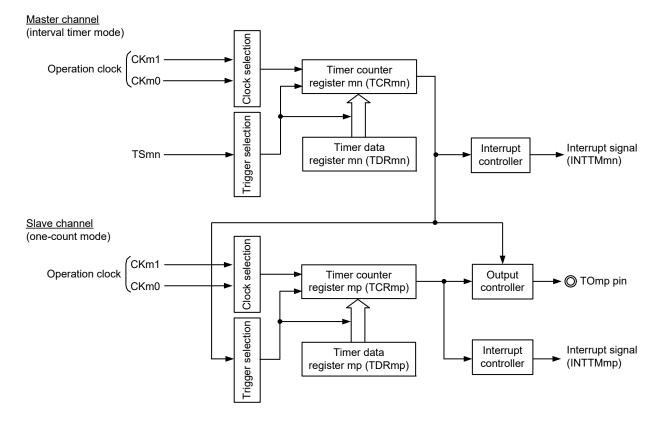
Figure 6 - 73 Block Diagram of Operation as PWM Function
