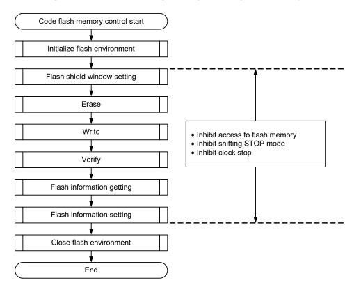
Figure 22 - 8 Flow of Self-Programming (Rewriting Flash Memory)
