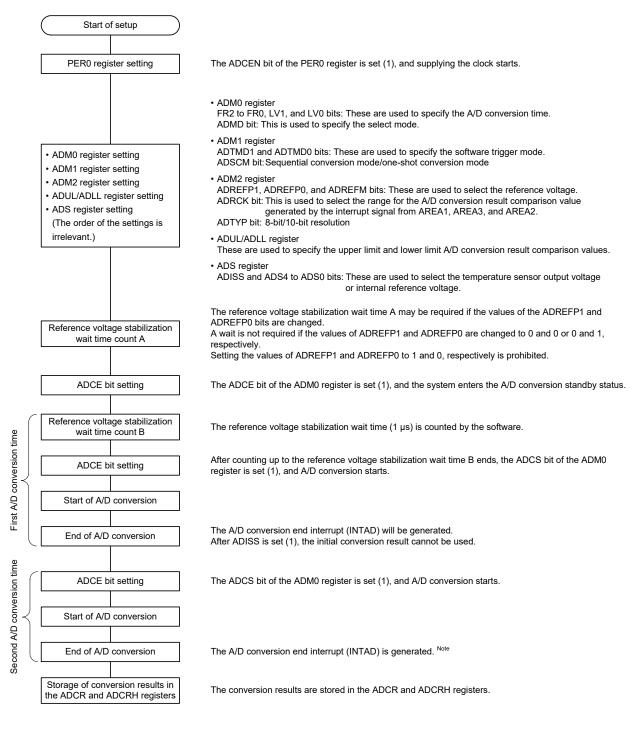
**Note** Depending on the settings of the ADRCK bit and ADUL/ADLL register, there is a possibility of no interrupt signal being generated. In this case, the results are not stored in the ADCR, ADCRH registers.
