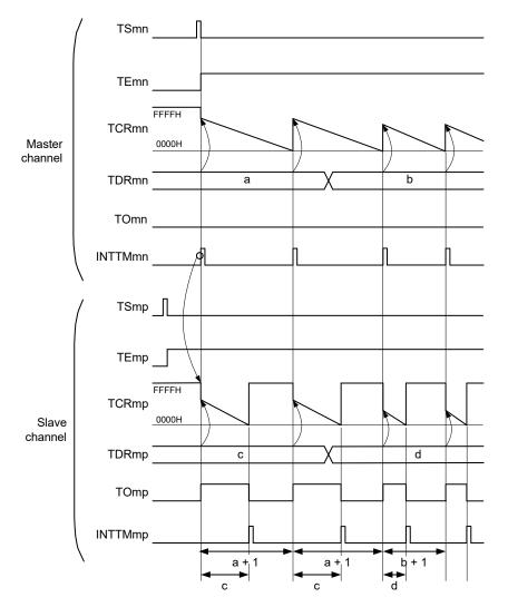
Figure 6 - 74 Example of Basic Timing of Operation as PWM Function
