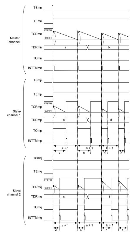
Figure 6 - 80 Example of Basic Timing of Operation as Multiple PWM Output Function (Output two types of PWMs) (1/2)
