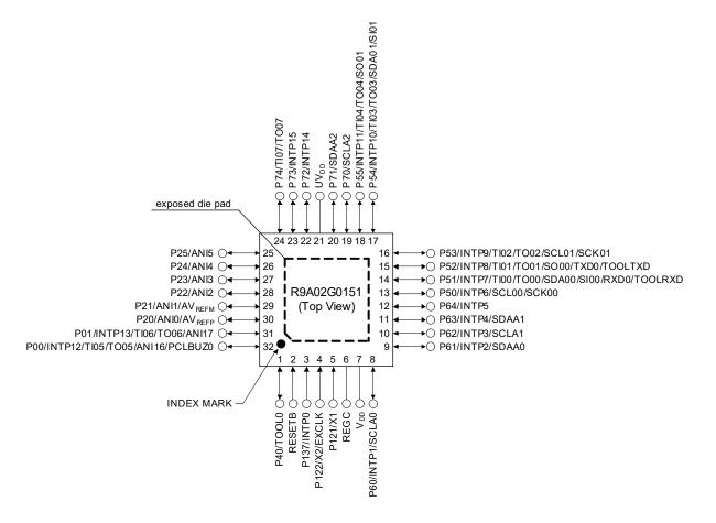
Caution 1. Connect the exposed die pad (Vss) to ground. Caution 2. Connect the REGC pin to Vss via a capacitor (0.47 to 1  $\mu$ F).
