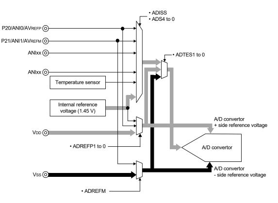
Figure 19 - 15 Configuration of A/D Test Function
