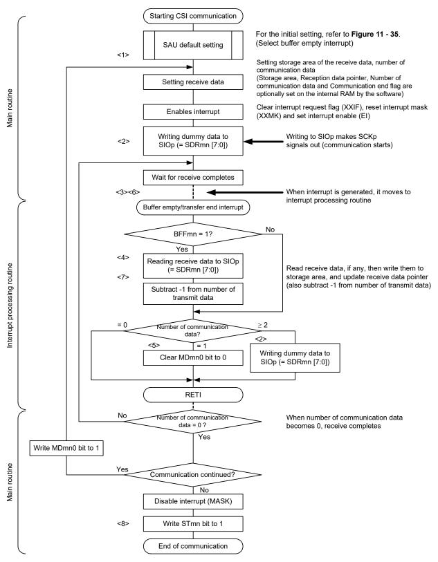
Figure 11 - 41 Flowchart of Master Reception (in Continuous Reception Mode)
