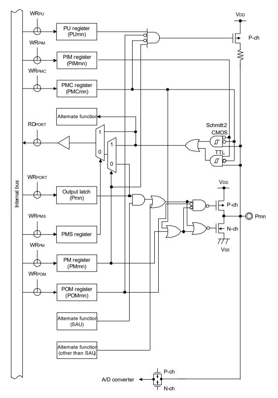
Figure 2 - 7 Pin Block Diagram of Pin Type 8-3-4
