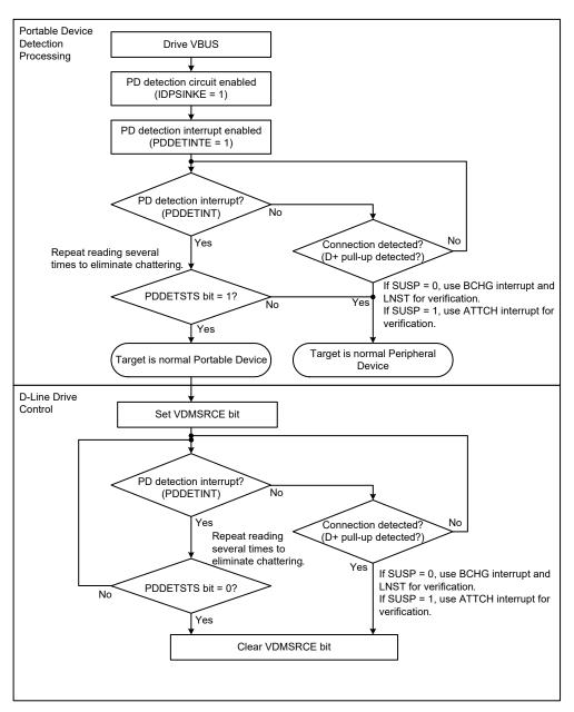
Figure 13 - 67 Process Flow for Operating as Charging Downstream Port (Steps (1) to (4))
