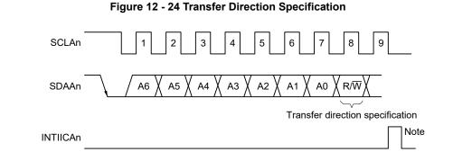
Note INTIICAn is not issued if data other than a local address or extension code is received during slave device operation.
