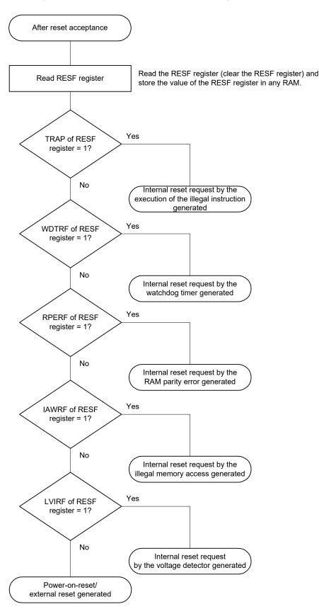
Figure 16 - 5 Example of Procedure for Checking Reset Source
