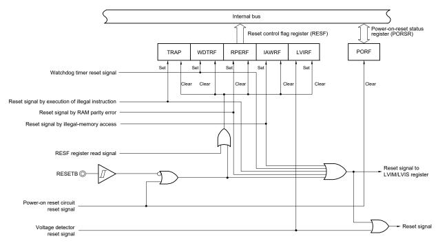
Figure 16 - 1 Block Diagram of Reset Function
