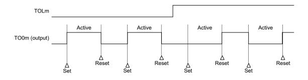
Remark 1. Set:The output signal of the TOmn pin changes from inactive level to active level.Reset:The output signal of the TOmn pin changes from active level to inactive level.
