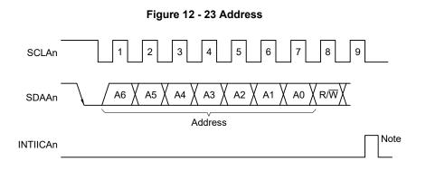
Note INTIICAn is not issued if data other than a local address or extension code is received during slave device operation.
