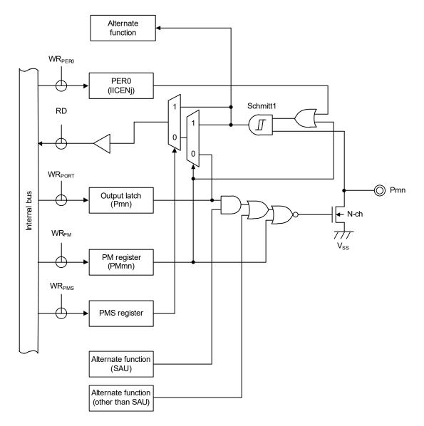
Figure 2 - 9 Pin Block Diagram of Pin Type 12-1-3
