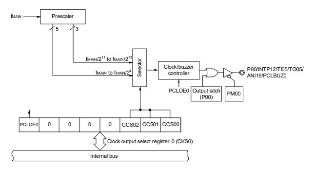
Figure 8 - 1 Block Diagram of Clock Output/Buzzer Output Controller
