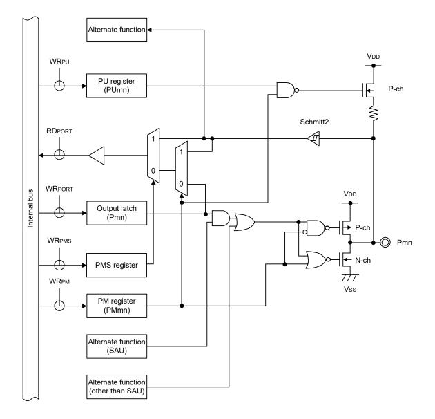
Figure 2 - 5 Pin Block Diagram of Pin Type 7-1-3
