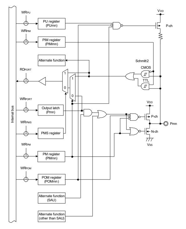
Figure 2 - 6 Pin Block Diagram of Pin Type 8-1-4
