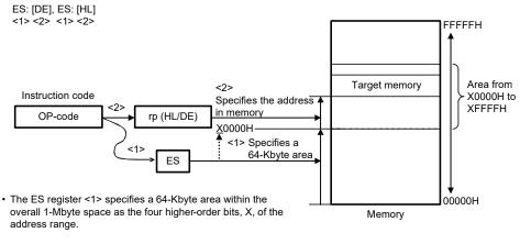
• Either pair of registers <2> and the ES register <1> specify the target location in the area from X0000H to XFFFFH.
