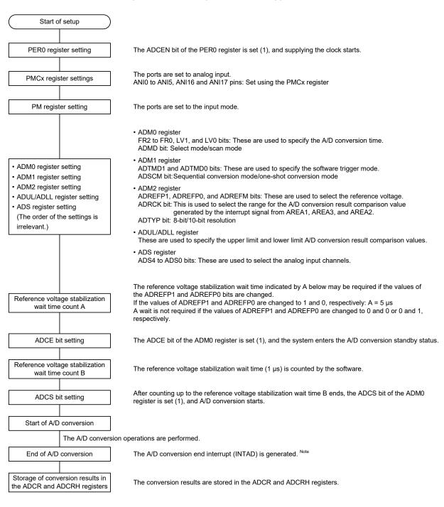
Figure 10 - 31 Setting up Software Trigger Mode
