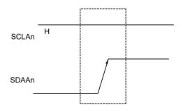
A stop condition is generated when bit 0 (SPTn) of IICA control register n0 (IICCTLn0) is set to 1. When the stop condition is detected, bit 0 (SPDn) of the IICA status register n (IICSn) is set to 1 and INTIICAn is generated when bit 4 (SPIEn) of the IICCTLn0 register is set to 1.
