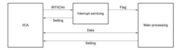
Therefore, data communication processing is performed by preparing the following three flags and passing them to the main processing instead of INTIICAn.
