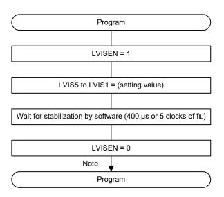
Figure 18 - 10 Changing of LVD Detection Voltage Setting
