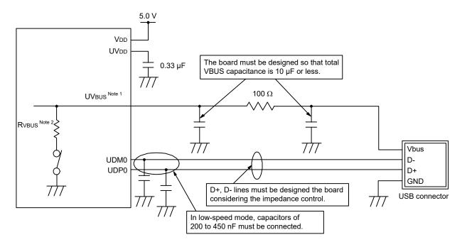
Figure 13 - 52 USB Connector Function Connection Example in Self-powered Mode (5 V)
