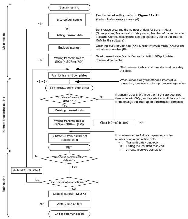
Figure 11 - 57 Flowchart of Slave Transmission (in Continuous Transmission Mode)
