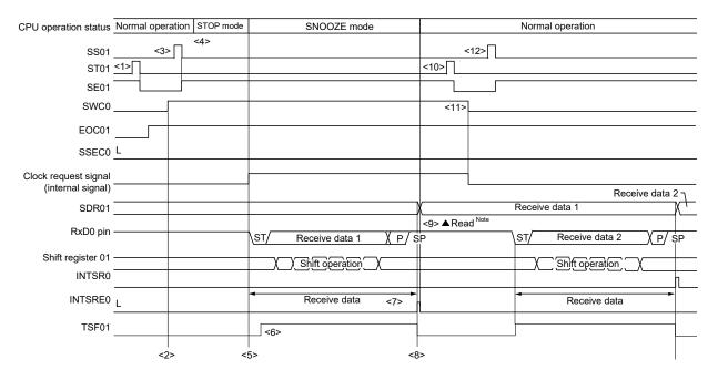
Figure 11 - 94 Timing Chart of SNOOZE Mode Operation (EOCm1 = 1, SSECm = 0)
