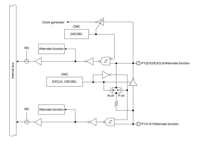
Figure 2 - 3 Pin Block Diagram of Pin Type 2-2-1
