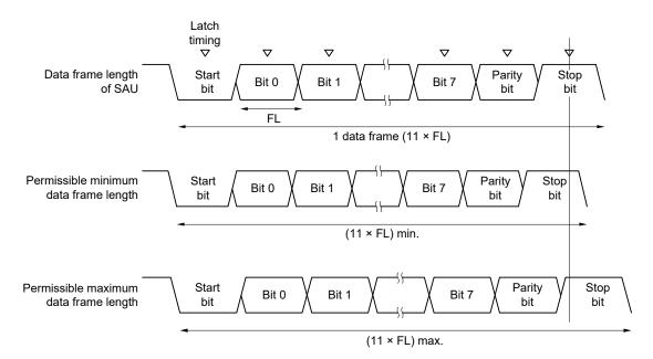
As shown in Figure 11 - 98, the timing of latching receive data is determined by the division ratio set by bits 15 to 9 of serial data register mn (SDRmn) after the start bit is detected. If the last data (stop bit) is received before this latch timing, the data can be correctly received.
