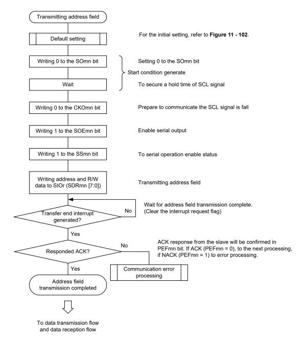
Figure 11 - 104 Flowchart of Address Field Transmission
