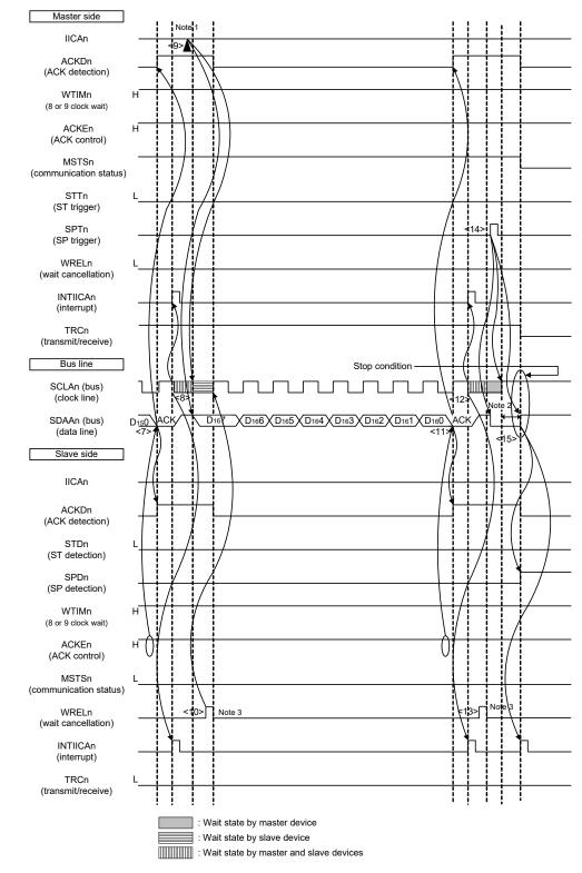
Note 1. Write data to IICAn, not setting the WRELn bit, in order to cancel a wait state during transmission by a master device.
