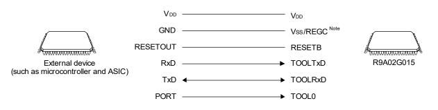
Note Connect REGC pin to ground via a capacitor (0.47 to 1  $\mu$ F).
