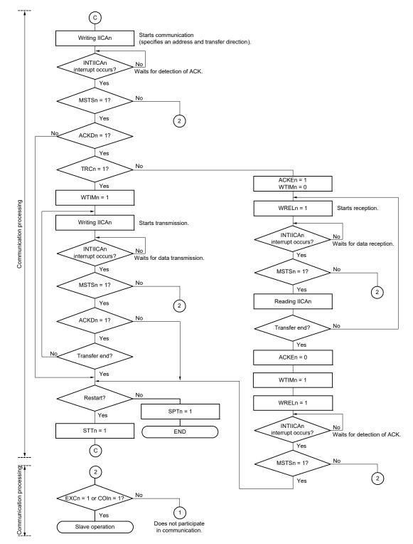
Figure 12 - 39 Master Operation in Multi-Master System (3/3)
