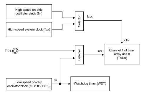
If pulse interval measurement results in an abnormal value, it can be concluded that the clock frequency is abnormal.
