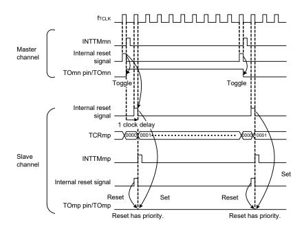
Remark 1.Internal reset signal:TOmn pin reset/toggle signalInternal set signal:TOmn pin set signalRemark 2.m: Unit number (m = 0)n: Channel numbern = 0 to 7 (n = 0, 2, 4, 6 for master channel)p: Slave channel numbern \leq 7
