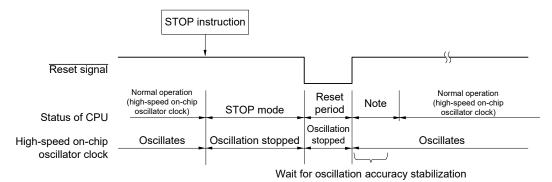
(2) When high-speed system clock is used as CPU clock
