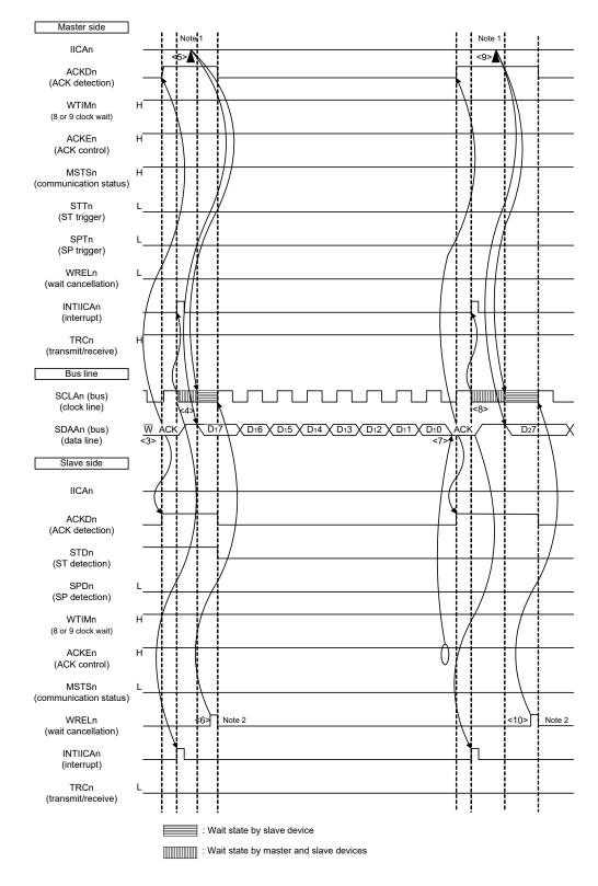
Note 1. Write data to IICAn, not setting the WRELn bit, in order to cancel a wait state during transmission by a master device. For releasing wait state during reception of a slave device, write "FFH" to IICAn or set the WRELn bit.
