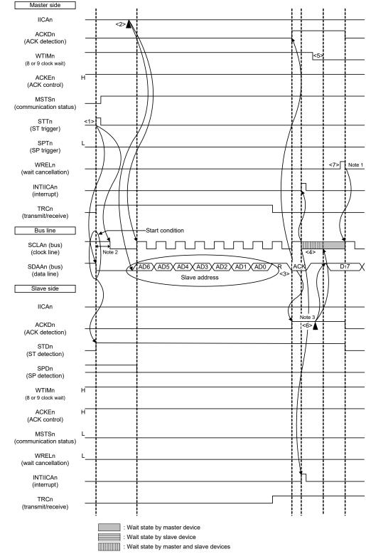
**Note 1.** For releasing wait state during reception of a master device, write "FFH" to IICAn or set the WRELn bit.
