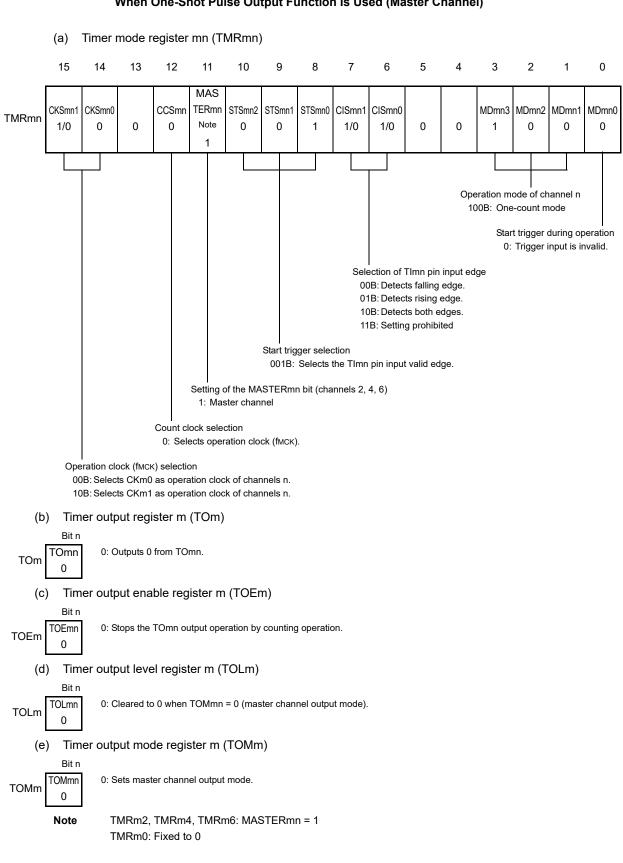
Figure 6 - 69 Example of Set Contents of Registers When One-Shot Pulse Output Function Is Used (Master Channel)
