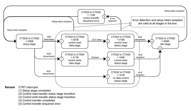
Figure 13 - 61 Control Transfer Stage Transitions
