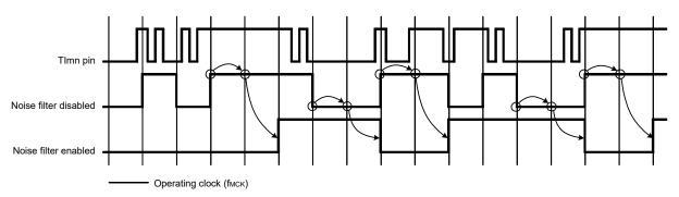
Caution The input waveforms to the Tlmn pin are shown to explain the operation when the noise filter is enabled or disabled.
