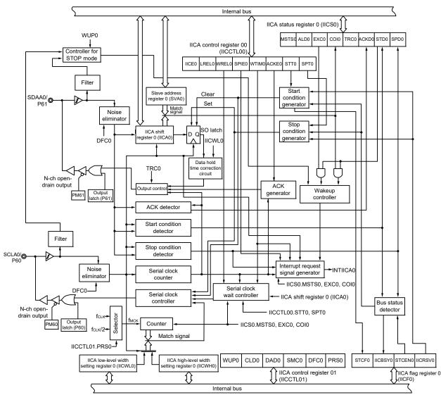
Figure 12 - 1 Block Diagram of Serial Interface IICA
