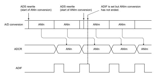
Figure 10 - 47 Timing of A/D Conversion End Interrupt Request Generation
