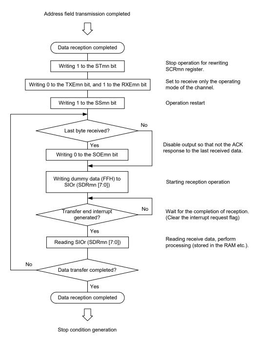
Caution ACK is not output when the last data is received (NACK). Communication is then completed by setting 1 to the STmn bit of serial channel stop register m (STm) to stop operation and generating a stop condition.
