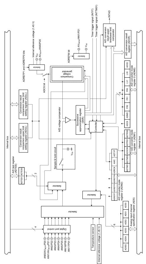
Figure 10 - 1 Block Diagram of A/D Converter
