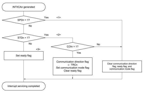
Figure 12 - 41 Slave Operation Flowchart (2)
