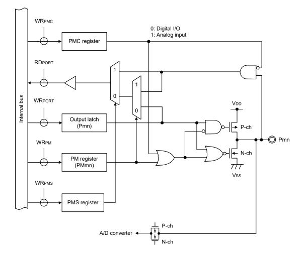
Figure 2 - 4 Pin Block Diagram of Pin Type 4-3-5
