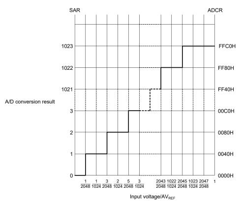
**Remark** AVREF: The + side reference voltage of the A/D converter. This can be selected from AVREFP, the internal reference voltage (1.45 V), and VDD.
