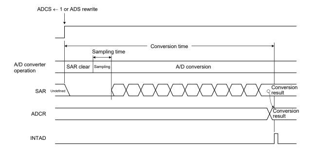
Figure 10 - 17 Conversion Operation of A/D Converter (Software Trigger Mode)
