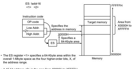
A 16-bit address <2> in the area from X0000H to XFFFFH and the ES register <1> specify the target location; this is used for access to fixed data other than that in mirrored areas.
