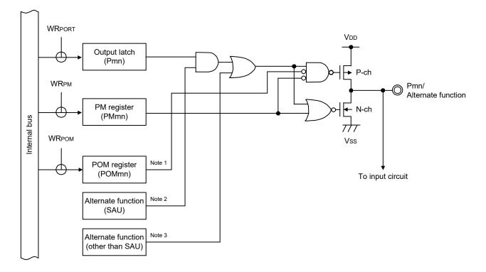
Figure 4 - 7 Basic Configuration of Output Circuit for Pins
