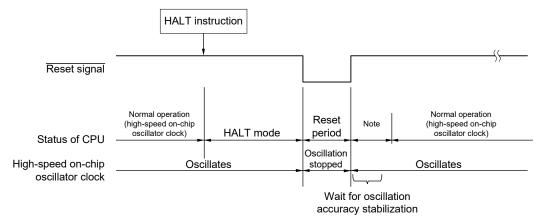
(2) When high-speed system clock is used as CPU clock
