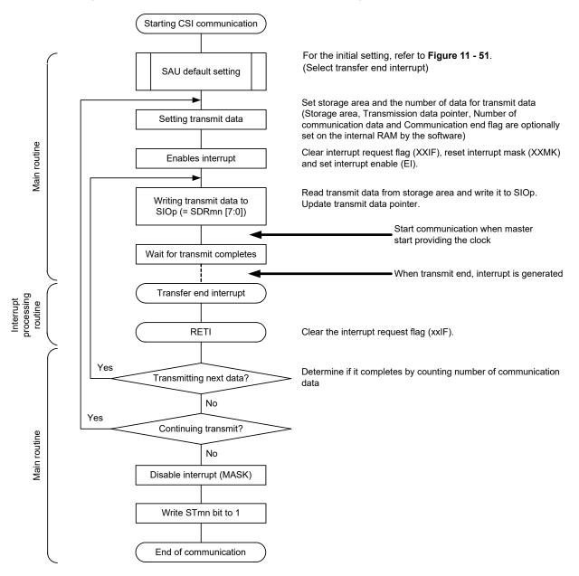
Figure 11 - 55 Flowchart of Slave Transmission (in Single-Transmission Mode)
