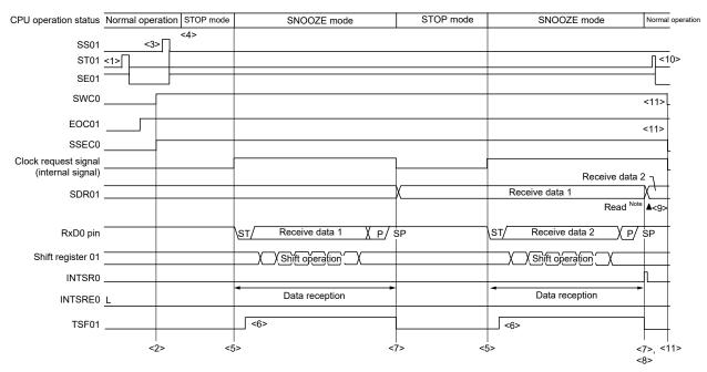
Figure 11 - 96 Timing Chart of SNOOZE Mode Operation (EOCm1 = 1, SSECm = 1)
