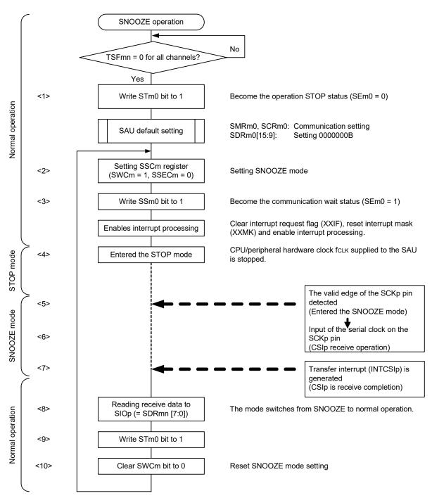
Figure 11 - 75 Flowchart of SNOOZE Mode Operation (continuous startup)
