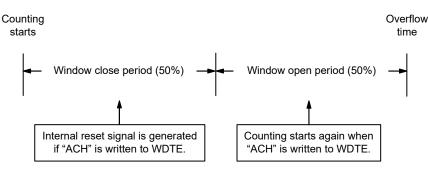
Caution When data is written to the WDTE register for the first time after reset release, the watchdog timer is cleared in any timing regardless of the window open time, as long as the register is written before the overflow time, and the watchdog timer starts counting again.
