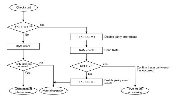
Figure 19 - 8 RAM Parity Error Check Flow
