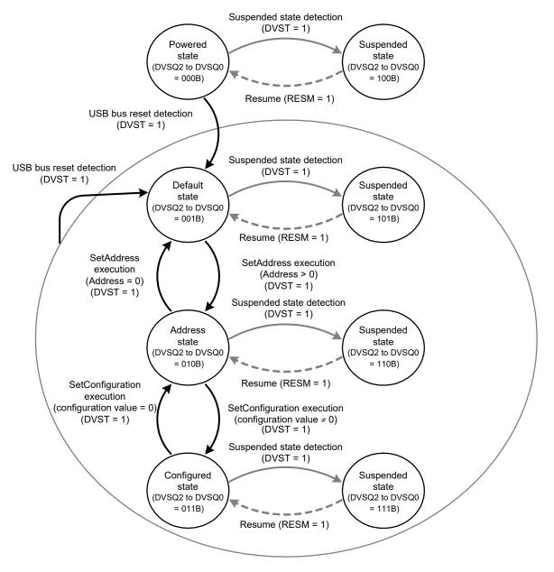
Figure 13 - 60 Device State Transitions
