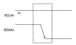
A start condition is output when bit 1 (STTn) of IICA control register n0 (IICCTLn0) is set (1) after a stop condition has been detected (SPDn: Bit 0 of the IICA status register n (IICSn) = 1). When a start condition is detected, bit 1 (STDn) of the IICSn register is set (1).
