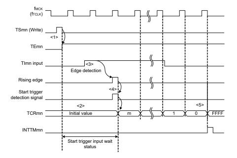
Figure 6 - 33 Operation Timing (In One-count Mode)
