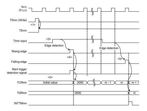
**Remark** The above figure shows the timing when the noise filter is not used. By making the noise filter on-state, the edge detection becomes 2 fMCK cycles (it sums up to 3 to 4 cycles) later than the normal cycle of TImn input. The error per one period occurs be the asynchronous between the period of the TImn input and that of the count clock (fMCK).
