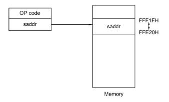
**Remark** SADDR and SADDRP are used to describe the values of addresses FE20H to FF1FH with 16-bit immediate data (higher 4 bits of actual address are omitted), and the values of addresses FFE20H to FFF1FH with 20-bit immediate data.
