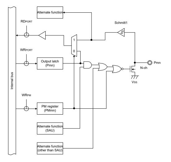
Figure 2 - 8 Pin Block Diagram of Pin Type 12-1-2
