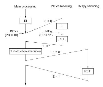
Interrupt request INTyy issued during servicing of interrupt INTxx is not acknowledged because its priority is lower than that of INTxx, and multiple interrupt servicing does not take place. The INTyy interrupt request is held pending, and is acknowledged following execution of one main processing instruction.
