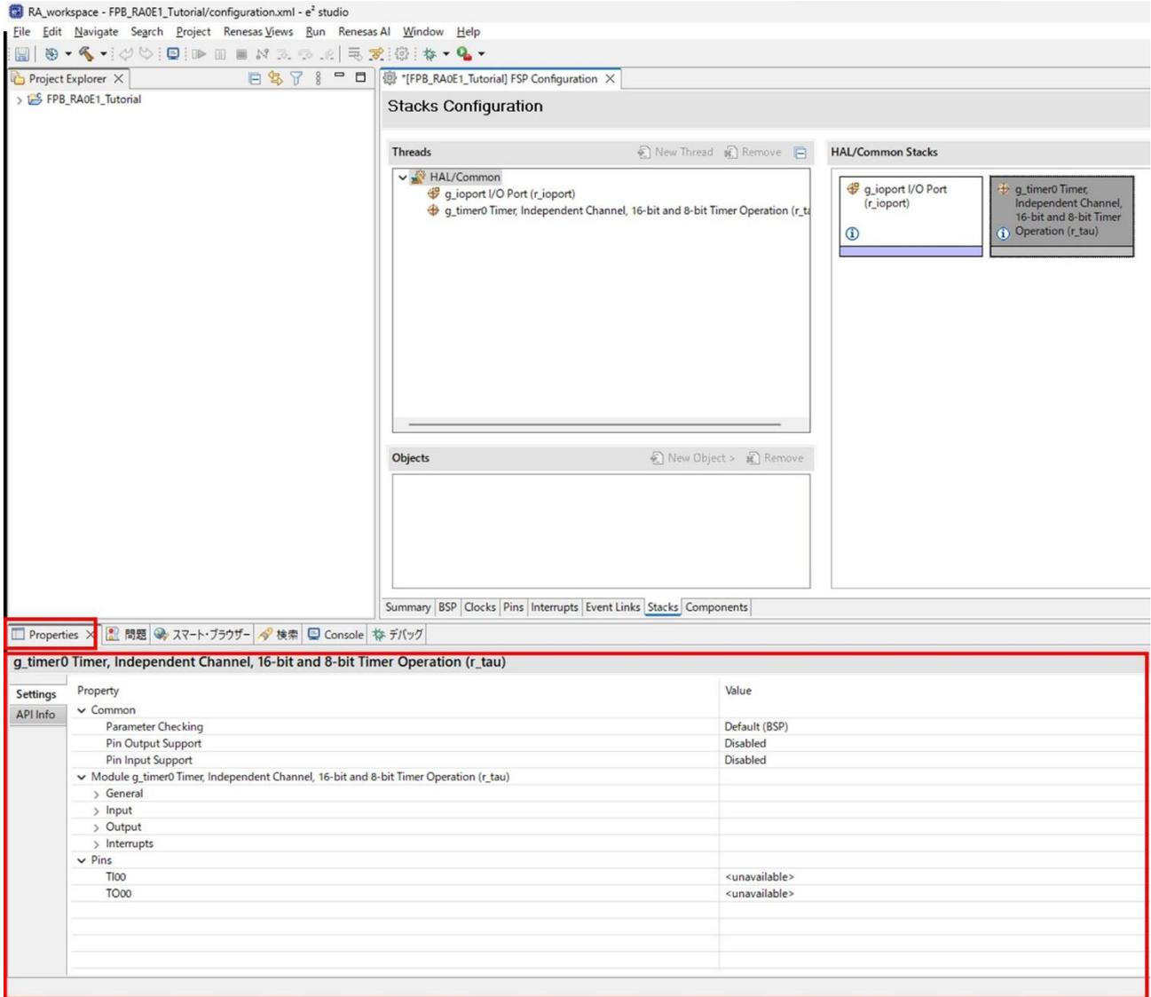
Figure 3-22 Setting the timer function
