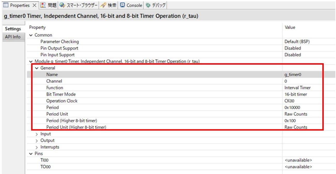
Figure 3-24 Setting the timer function
