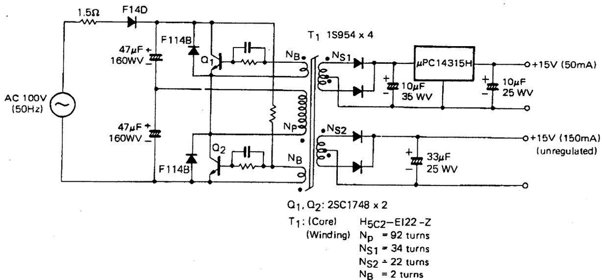
Figure 10. Schematic Diagram of Half-Bridge Type DC-DC Converter
