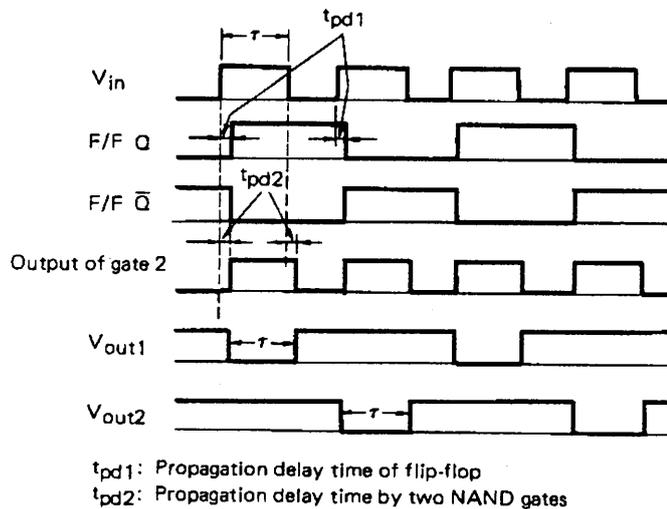
**Figure 7. Operating Waveform of Two-Phase Clock Circuit**
