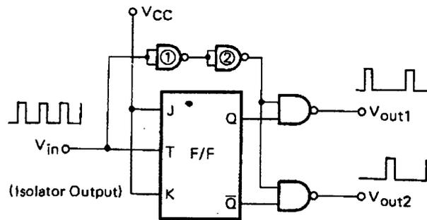
**Figure 6. Two-Phase Clock Circuit**
