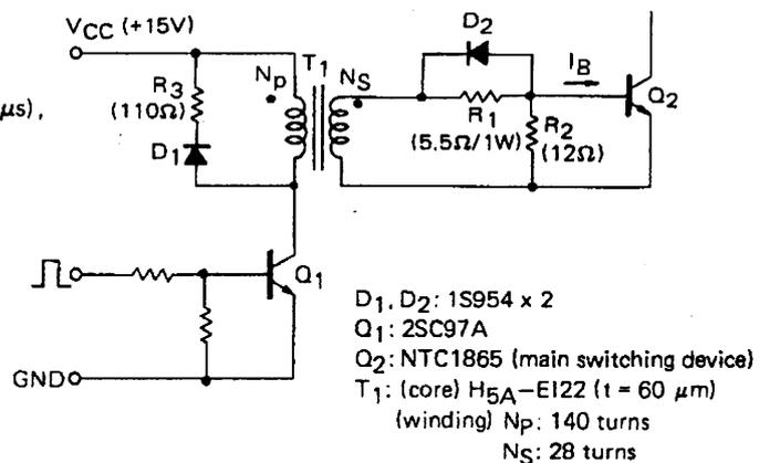
Figure 11. Base Driving Circuit
