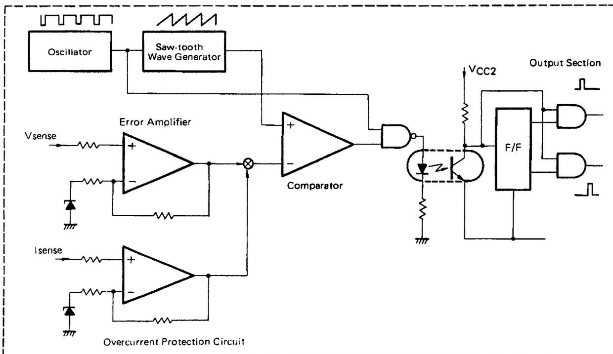
Figure 1. Block Diagram of Control Circuit
