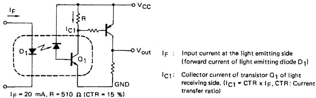
**Figure 5. Isolator Circuit using High Speed Photocoupler**
