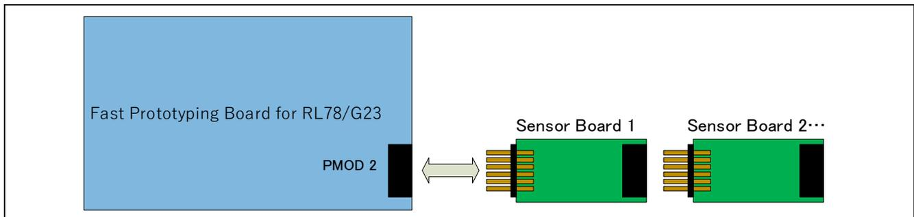
Figure 2-4 Hardware Connections for the RL78/G23 Group
