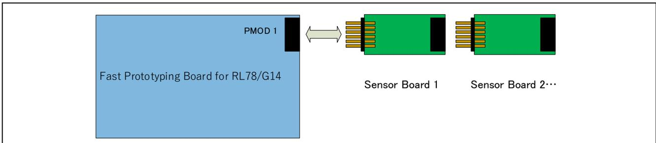
Figure 2-3 Hardware Connections for RL78/G14 Group
