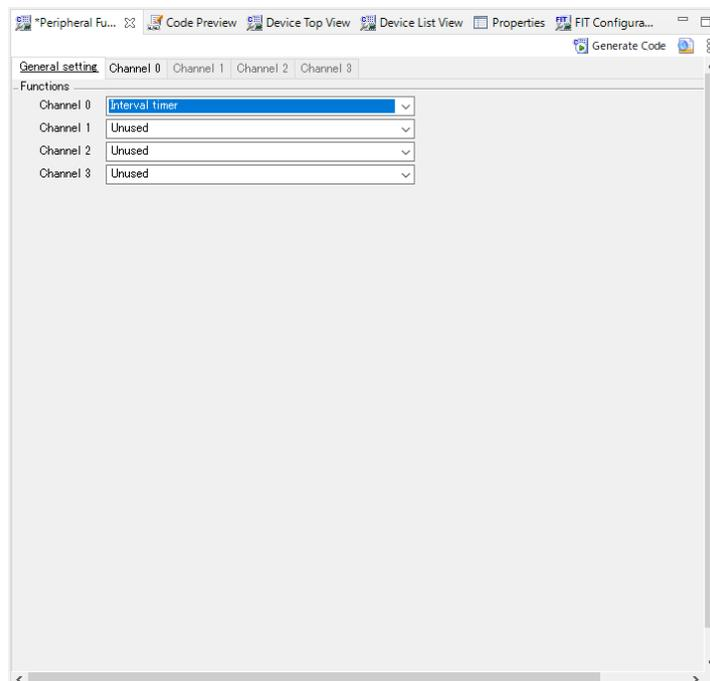
In the page for the channel set to the interval timer, set "Interval value" to "100  $\mu$ s", enable timer interrupts, and set the interrupt priority to a desired level.
