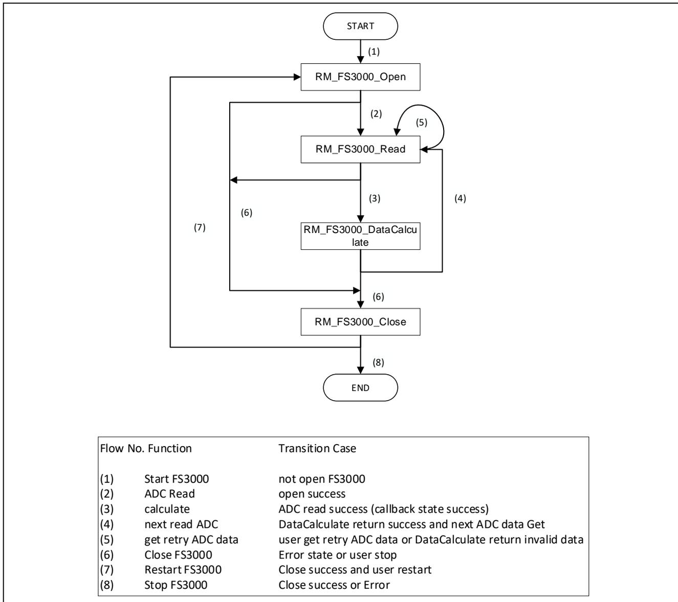
Figure 4-2 Diagram of Transitions between API Function Calls
