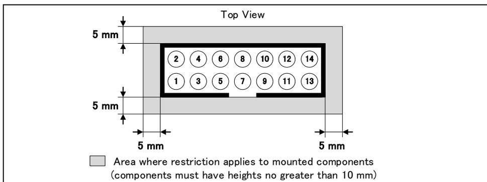
Figure 2-1 Area where Restriction Applies to Mounted Components
