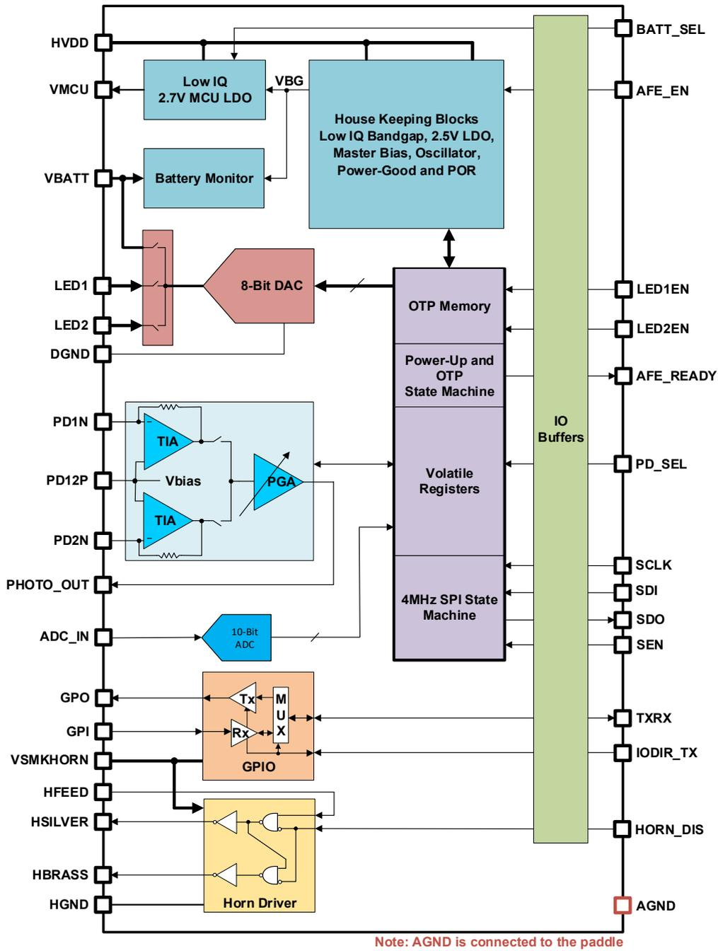
Figure 2. Block Diagram
