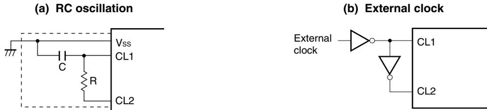
**Caution** When using the system clock oscillator, wire as follows in the area enclosed by the broken lines in Figure 5-10 to avoid an adverse effect from wiring capacitance.
