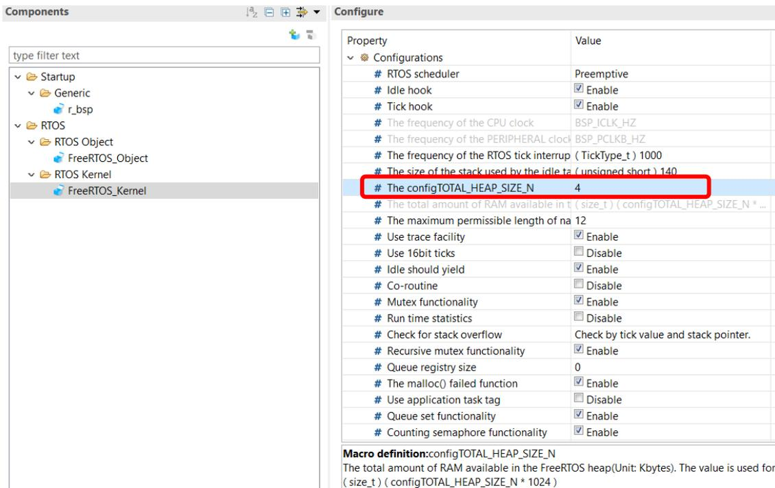
Total allocated RAM size is calculated with the following expression: (configTOTAL\_HEAP\_SIZE\_N\*1024).
