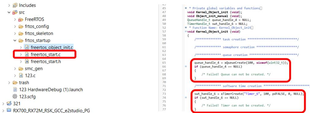
Heap usage of modified objects will be displayed in “Total Amount Heap Usage” group after code generation. Object heap usage exceeding the total available heap space will result in build error.
