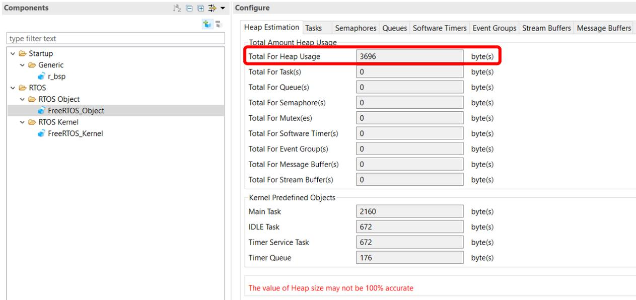
The macro “configTOTAL\_HEAP\_SIZE\_N” in FreeRTOSConfig.h is used to set the total available heap space. This macro can be modified by changing “The configTOTAL\_HEAP\_SIZE\_N” configuration in FreeRTOS\_Kernel as shown in the following picture:
